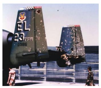
Damaged tail section of Dave Sawyer's A-10 aircraft after being struck by an Iraqi rocket. Courtesy of Jeanne Sawyer
