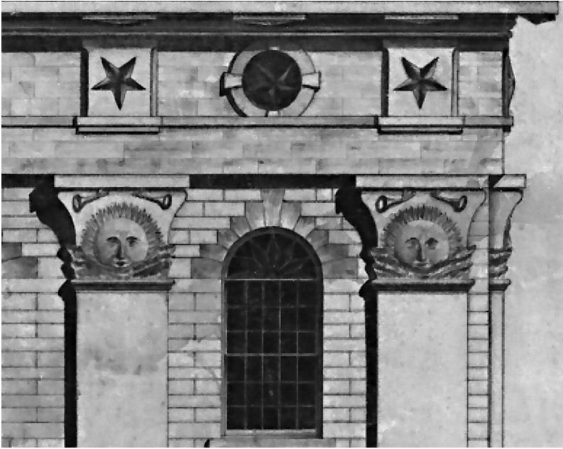
Figure 2. Portion of what was likely the final architectural drawing by William Weeks of the front of the Nauvoo Temple showing two “full-faced” sunstone capitals on the pilaster, circa 1841–46. Church History Library.
