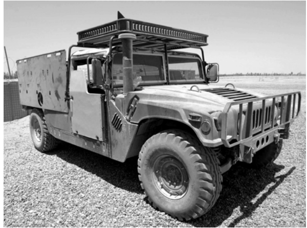
This HMMWV—pictured near Camp Fallujah, Iraq, in July 2004—has an ERC (explosive resistant coating) armored door to better protect the occupants. Courtesy of DoD.
